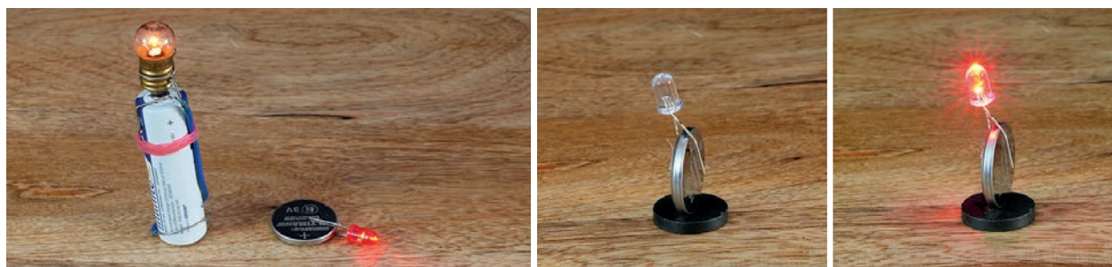
Fig. 1.10 On the left: Simple circuits. On the right: A button cell standing on a magnet, with the shorter leg of an LED taped to the negative terminal. The LED lights up when the bent leg touches the positive terminal.
